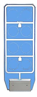
This **Hybrid** (**UHF RFID + EM**) **security gate system** is used to detect the books using method of SECURITY BIT and EM detection which are passing through the gates. There are 2 types of frequency for these gates, which are UHF (902MHz-928MHz) and EM (1kHz). If any of the security bits or the EM strips of the books are still activated, the alarm of the gate will be alerted when the books are passing through the gate.
