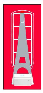
This **Hybrid** (**UHF RFID + EM**) **security gate system** is used to detect the books using method of SECURITY BIT and EM detection which are passing through the gates. There are 2 types of frequency for these gates, which are UHF (902MHz-928MHz) and EM (1kHz). If any of the security bits or the EM strips of the books are still activated, the alarm of the gate will be alerted when the books are passing through the gate.
